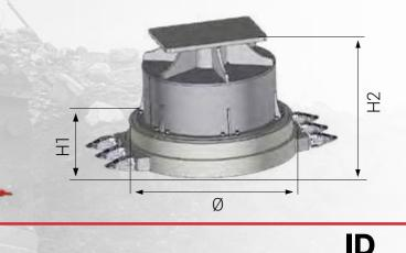
Hydraulic electromagnets with teeth are mainly used in demolition sites. The teeth are designed to rake debris, making it easier to extract ferrous materials. Theeth are also equipped with a quick fitting device and are easy to replace in case of wear. These electromagnets are equipped with a plate for quick hitch, providing the advantage that they can be attached without manual intervention. They are typically used with excavators and heavy machinery due to their high weight.
