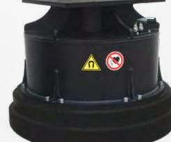
Hydraulic electromagnets with a plate for quick coupling can be attached without operator's manual intervention and have a more precise positioning on the material, making them extremely efficient. In addition, the plate can be modified/customised according to customers needs, in order to fit the used machinery. They are typically attached to excavators.
