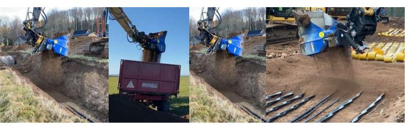
The MAX range is known for the longer wider cutting edge. These systems have the largest capacity buckets in the Gyru-Star range holding up to 1.60m<sup>3</sup>. The specialist design makes material easier to pick up and makes them perfect for padding and backfilling.
