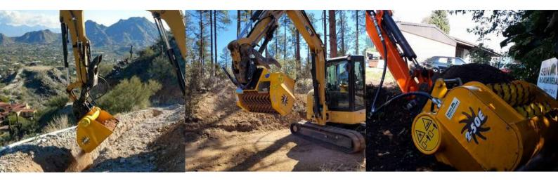
The E Range are the smallest screening systems available in the Gyru-Star Compact Screening family. These systems are suitable for excavators ranging from 1-5 ton. Perfect for work areas where space is limited. There are three fragment sizes to choose from and interfaces are also available.
