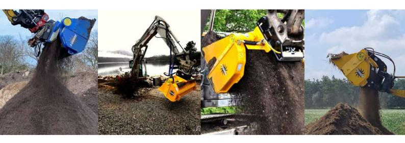
The Compact Screening Systems in the HDX Range are 1500mm wide and have additional hardox wear plates. The unique design of this range allows for loader conversion and when used in conjunction with a Kustom Konnect interface, the systems can have a dual interface system.
