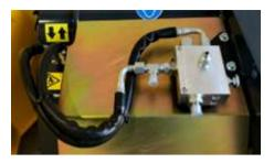
**Oil Flow Control** to control oil flow speeds.
