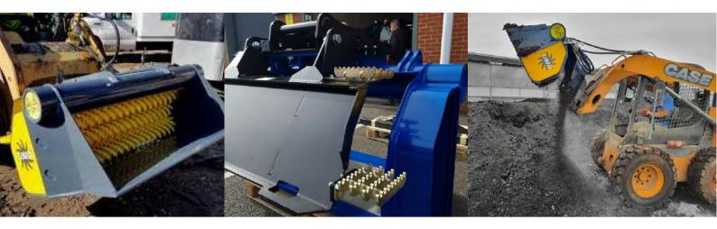
The SL range is our dedicated range for skid steer loaders. The unique design allows safe entry to the cab via integrated steps. These models have rotors varying from 1200mm to 1500mm in width.
