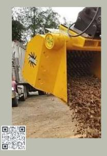
**4-100HE** 4 Rotors 1000mm Wide 7-10 ton Excavator 0.35m<sup>3</sup> Capacity
