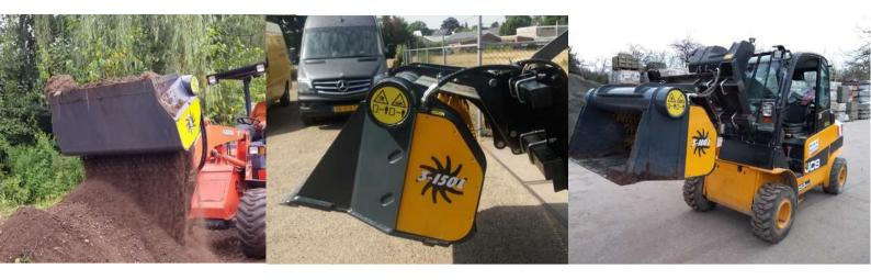
The L range is our dedicated range for loaders. The specialist shell design allows dedicated Kustom Konnect interfaces to added for easy carrier connection. This can be fixed, adjustable or interchangeable to suit your carrier needs.
